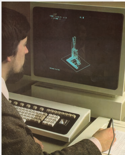
A model of a process plant being interactively designed in PDMS.
