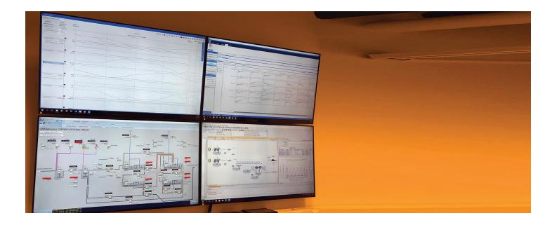
To understand and operate the plant, Oulu worked with AVEVA and Schneider Electric to implement the same software and controls tools used by most of the world's largest metals, mining and minerals companies. Students use DYNSIM Dynamic Simulation and advanced process control tools to bring to life the algorithms and technologies behind the real process. Students can simulate the process before running it to understand how theoretical models translate to real world implementation.
