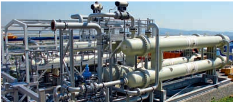
AVEVA PDMS model of a heat exchanger unit for the Beregovoye gas condensate field project. Image courtesy of RGE.
