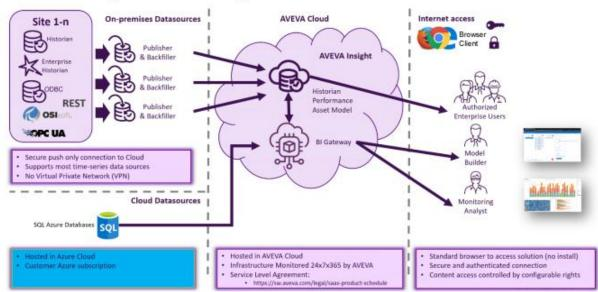
The above diagram shows that AVEVA Insight BI Gateway Module is a module that primarily leverages data from the various AVEVA Insight structures (time-series, performance, assets, etc). Optionally, this can be complemented by another SQL Azure data source. Users can then use their favorite BI tool to access the data store created by AVEVA Insight BI Gateway Module on Microsoft SQL Azure, for monitoring purposes.
