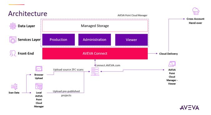
AVEVA Point Cloud Manager has a server-less architecture using compute functions to access content held in cloud storage and document databases.
