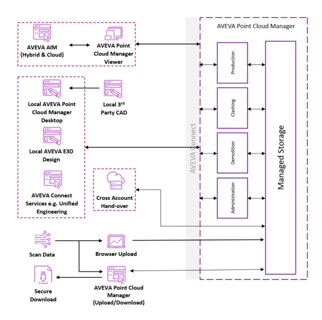
AVEVA Point Cloud Manager is a multi-tenanted application with a serverless architecture that uses compute functions to access content held in cloud storage and document databases.
