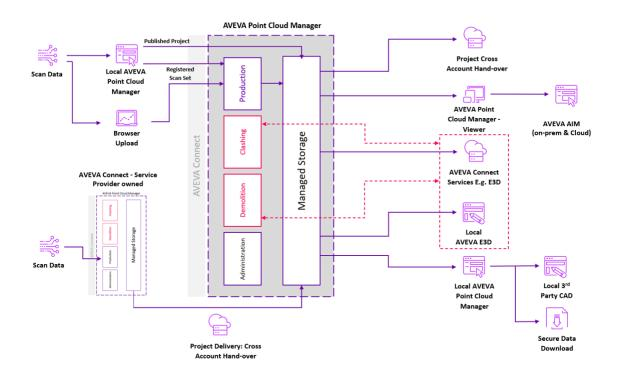
AVEVA Point Cloud Manager has a server-less architecture using compute functions to access content held in cloud storage and document databases.
