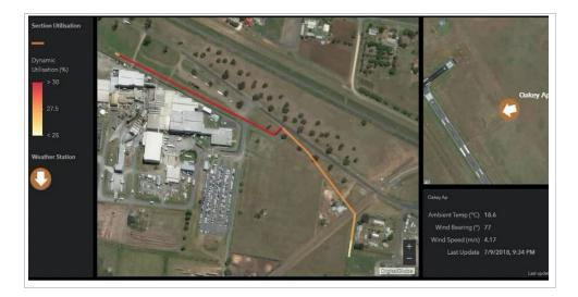
Integration of the PI System with Esri ArcGIS reveals the dynamic load on a segment of power line in real time. Segments that are more parallel to the direction of the wind retain more heat and have less excess power-carrying capacity than more perpendicular segments.
