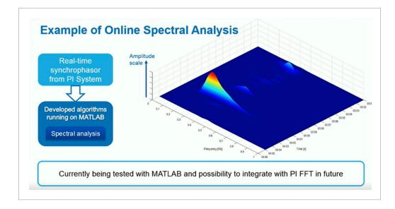
Disturbances or oscillations shown by online spectral analysis help control center operators identify when there are problems in the power system.
