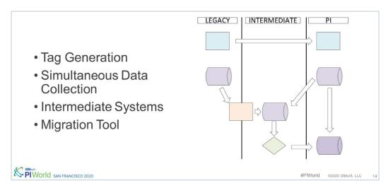
To migrate Genentech's historical data from a legacy system, consultant RoviSys used two AVEVA PI System installations, migrating and validating data in an intermediate system before registering it to the live server
