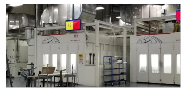
PI Vision displays with color-coded alarms help to monitor temperature and humidity in real time inside the paint booths for drones.
