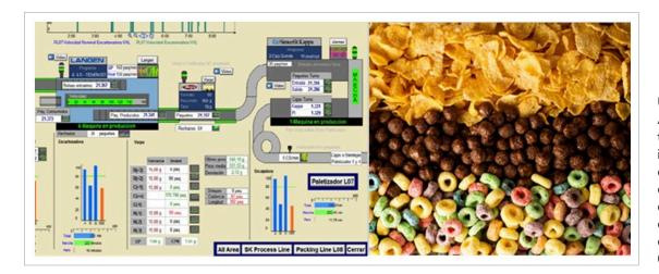
Using the PI System's Asset Framework, the Kellogg's plant in Valls, Spain, has created a digital twin of plant operations and increased overall equipment effectiveness from 67% to 80%.
