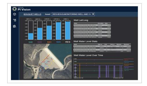
AVEVA PI Vision dashboard helps the LAPWD monitor the health of its dams at the Bouquet Reservoir in California by displaying important information about water levels in wells beneath the dams.
