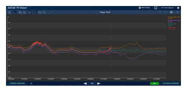
Methanex uses a generative pre-trained model designed for time series forecasting and anomaly detection to forecast steam turbine discharge pressure at one of its sites.
