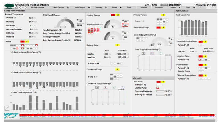
Entire CP6 building dashboard showing key parameters of CHW production, chilled water flow, condenser pumps, primary pumps, secondary pumps, tertiary pumps, cooling towers and chiller
