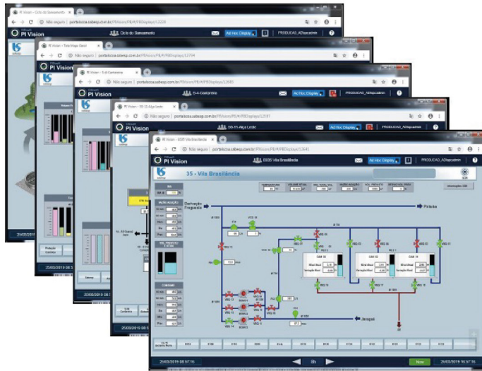
Using AVEVA PI Vision, Sabesp monitors various components of its water production infrastructure.
