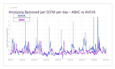
AVEVA APC improved process control and removed ammonia more efficiently from wastewater than SPR's ABAC model
