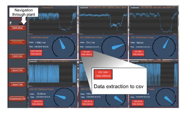
Toyota's PI Vision navigation dashboard allows for intuitive access to data across multiple sites, giving engineers insight into gas, electricity, and compressed air usage.
