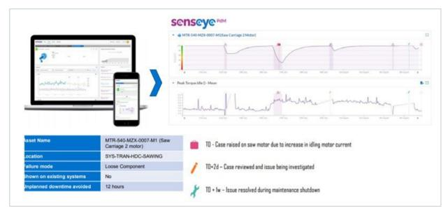
With event frames in AVEVA PI Server, Alcoa was able to track down anomalies during the runtime of the saw that were previously undetectable by the maintenance team, and avoid twelve hours of unplanned downtime
