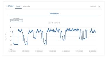
This dashboard shows energy production from fuel cells, indicating an excess of net metering on the weekends.
