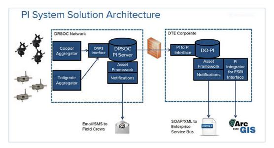
DTE Energy used fault sensors and AVEVA PI System to monitor outages on its power grid and provide field crews with real-time data on outages so they could restore service to customers quickly and efficiently
