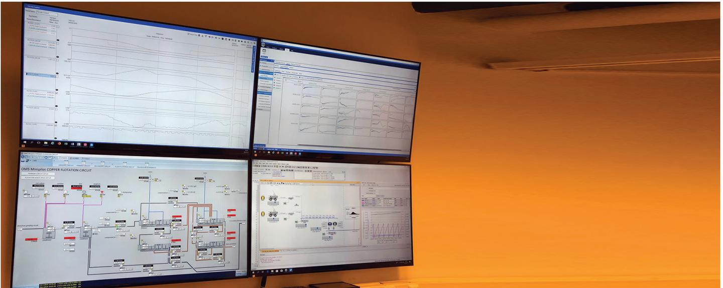
To understand and operate the plant, Oulu worked with AVEVA and Schneider Electric to implement the same software and controls tools used by most of the world's largest metals, mining and minerals companies. Students use DYNASIM Dynamic Simulation and advanced process control tools to bring to life the algorithms and technologies behind the real process. Students can simulate the process before running it to understand how theoretical models translate to real world implementation.
