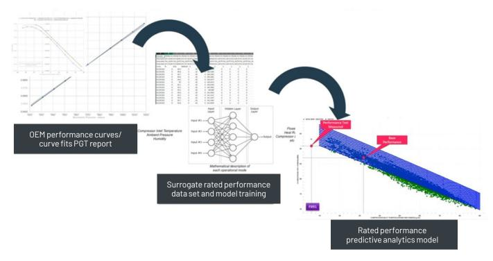
Suncor used AVEVA Process Optimization machine learning capabilities to analyze OEM performance curves and develop a rated model that could provide an accurate benchmark for gas turbine performance degradation
