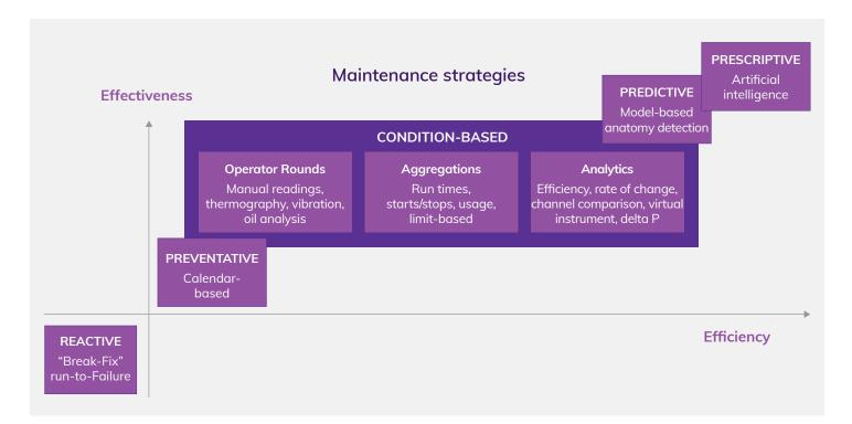
Reactive maintenance is necessary when equipment breaks down but can be a costly process, leading to downtime, which affects productivity. Preventative maintenance will help improve asset reliability, but there will still be unplanned downtime and costly repairs that could have been avoided with a more efficient method. Even regularly scheduled preventative maintenance is inefficient because 82% of machine failures occur at random intervals.<sup>3</sup>
