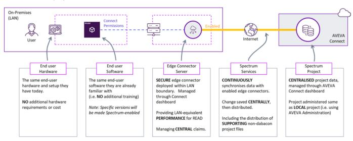
Applications such as AVEVA E3D run on the user's desktop at their location, accessing databases and project data through Spectrum services running on the edge connector. When a user saves data, changes are written to cloud-hosted Spectrum storage by the client application, which in turn triggers the edge connector caches at all locations to be updated. Various other metadata services are also hosted in AVEVA Connect.
