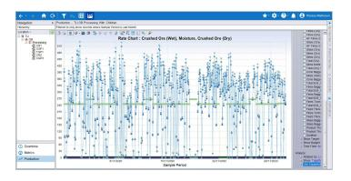
The visualization layer provided by the application's user interface allows users to easily drill down and determine the root causes, categorizing via Pareto or pie charts, the frequency and duration of all production-related losses.
